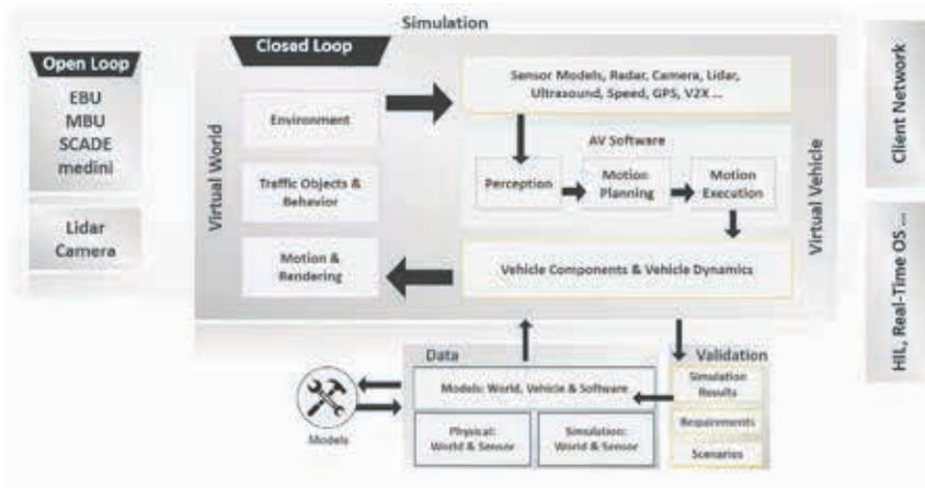
Figure 6. Illustration of the Ansys comprehensive solution for simulating autonomous vehicles miles driven.
